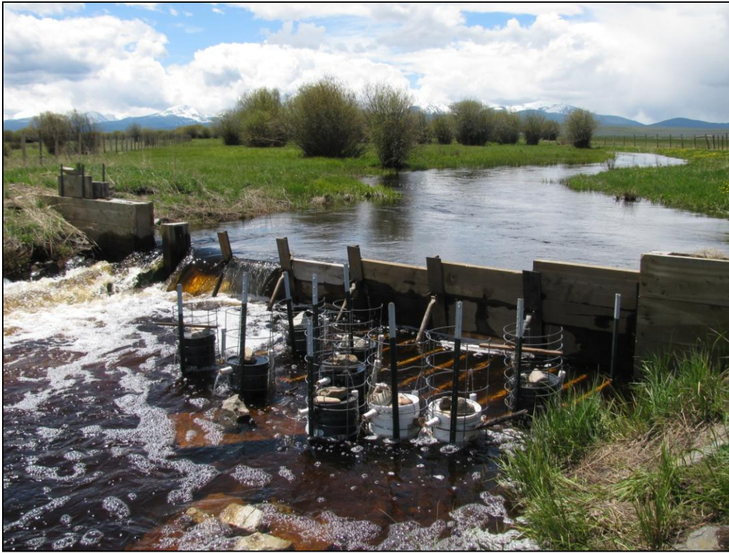
Figure 9. Remote site incubators were positioned downstream of existing pin and plank diversion structure to alleviate high flow conditions and provide backwater areas for emerging fry.
