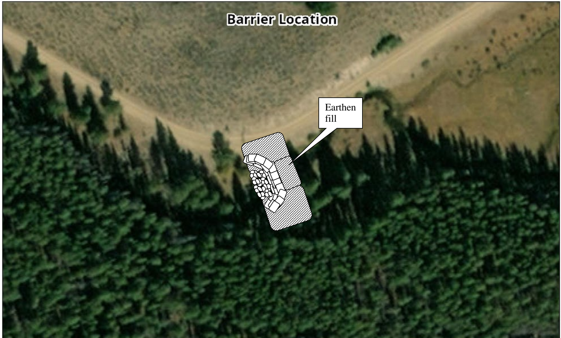
Figure 2. Drawing of the proposed fish barrier on Andrus Creek (not to scale) showing the earthen berm and rock spillway. Flow of Andrus Creek is right to left on the photo.
