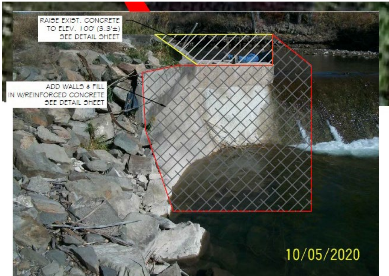
Figure 3. Conceptual approach of retrofit planned to block passage of rainbow trout.
