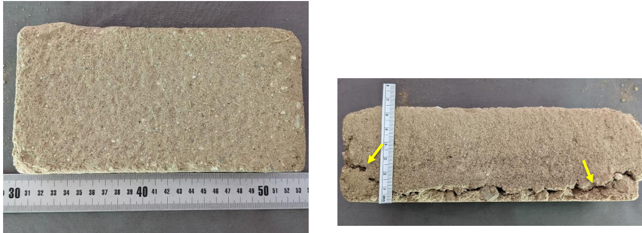
Figure 8: Replica adobe brick sample. Arrows in the side view of the sample, on right, show a region of poor consolidation.
