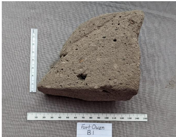
Figure 5: B1 Original adobe brick sample.
