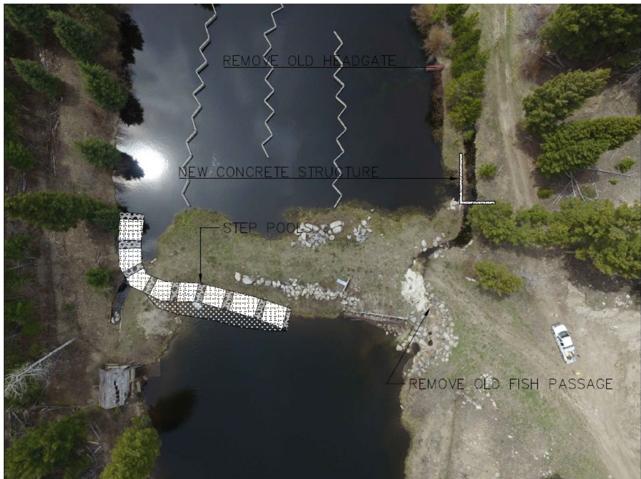
Figure 5. Design drawings of new fish passage channel that will connect South Fork Reservoir to the creek upstream.
