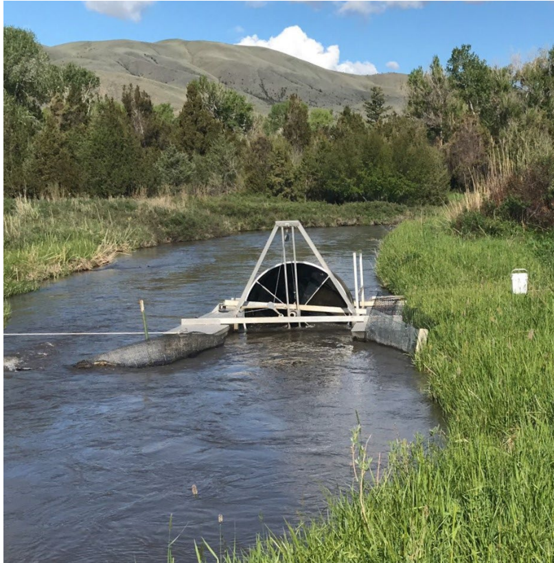
Figure 28. Rotary screw trap used to monitor fish outmigration from Deep Creek.
