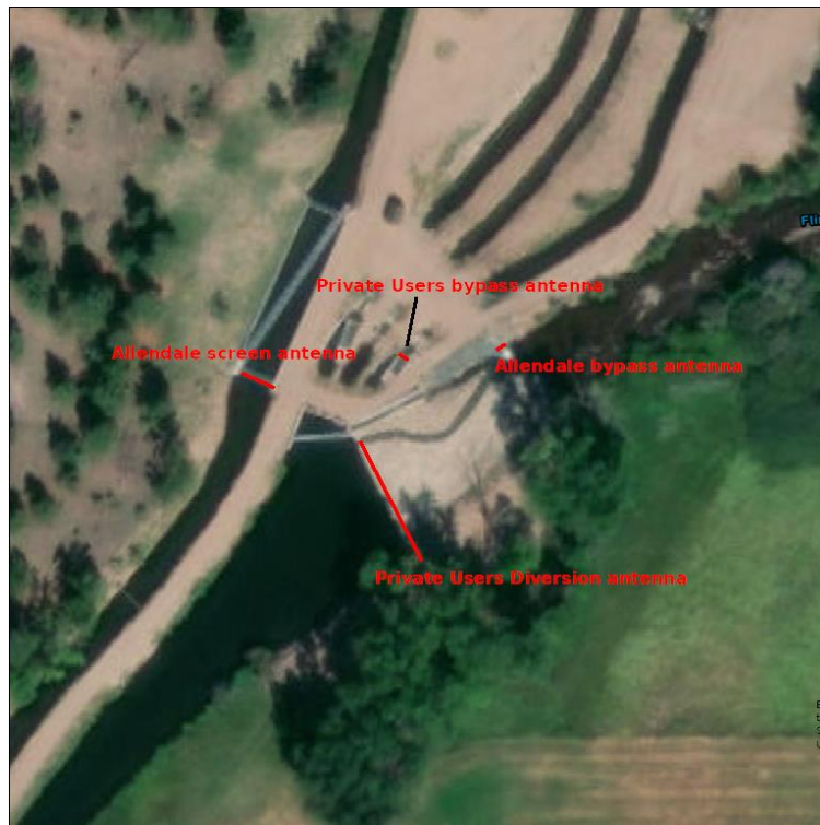
Map 4. Location of the PIT antenna pair near the town of Hall. Multiple antennae are used to gain directionality of fish movement. This site was used as a midway check point between the Allendale and Private Users fish screens and the mouth.
