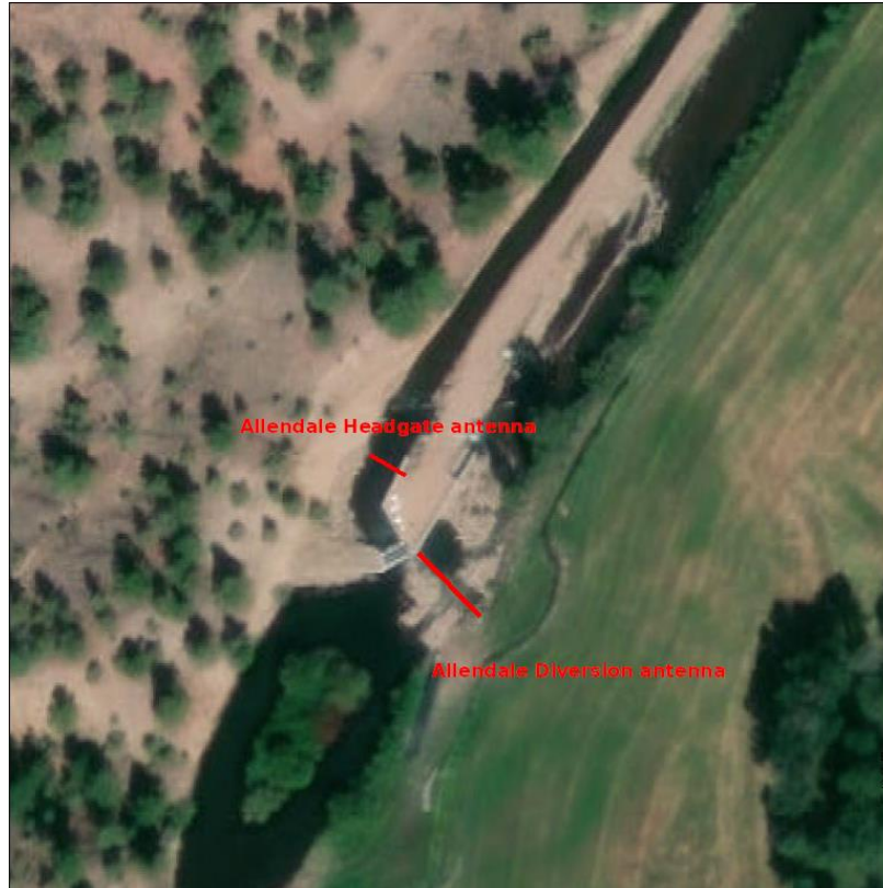
Map 6. Locations of PIT antennae around the Allendale diversion structure.
