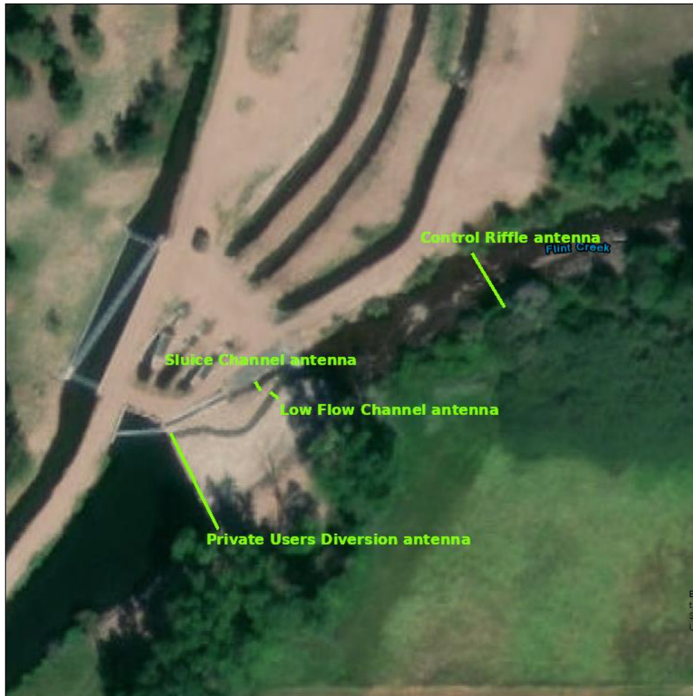
Map 7. Location of PIT antennae used to assess fish passage over the Private User's Diversion.
