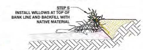
3 RECOMMENDED VEGETATED WOOD MATRIX INSTALLATION SEQUENCE 1" = 5'
