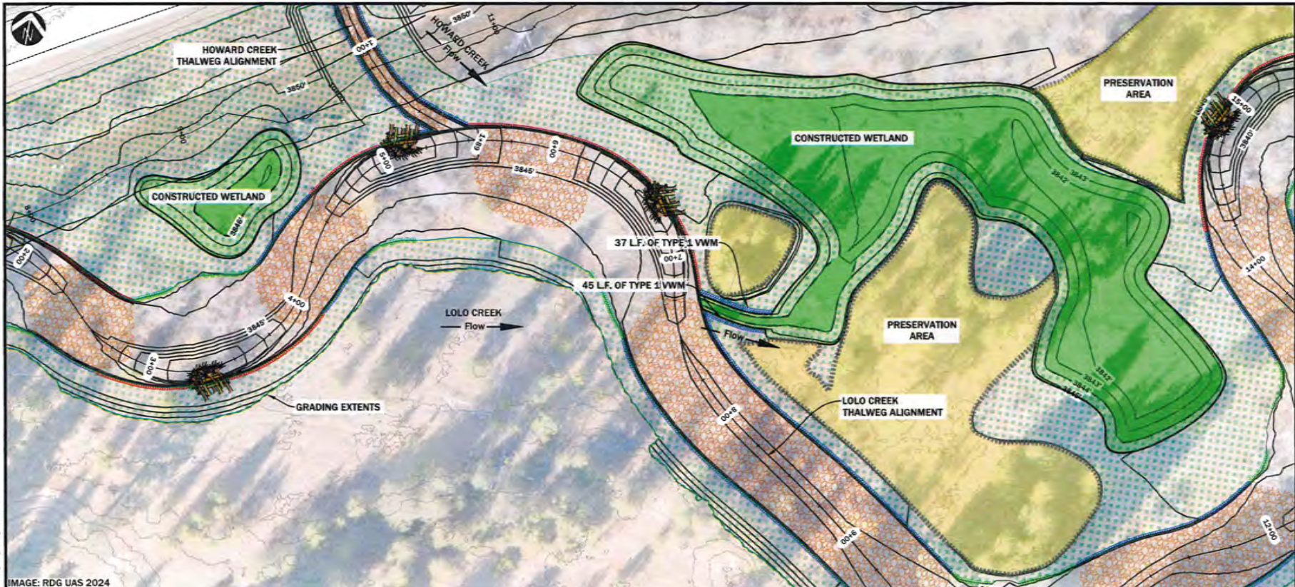
1 WETLAND CONSTRUCTION PLAN PLAN VIEW 1" = 50'
