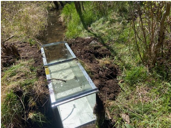
Figure 6. Temporary ditch flow measurement flume installed in Gratton Ditch in 2022, flow measured at 1.5CFS
