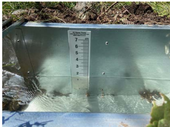
Figure 6. Temporary ditch flow measurement flume installed in Gratton Ditch in 2022, flow measured at 1.5CFS
