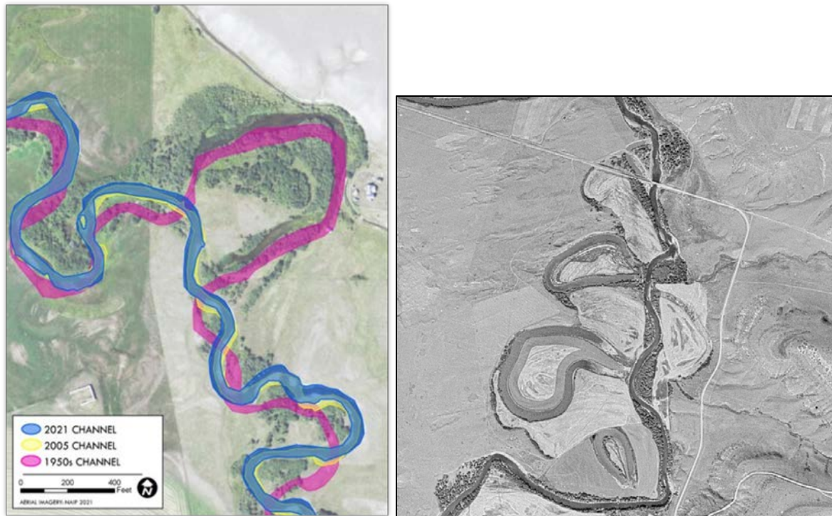
Figure 49. Example of channel adjustments over time (left) and pre 1950s meander cutoffs in agriculture area in lower watershed (right).
