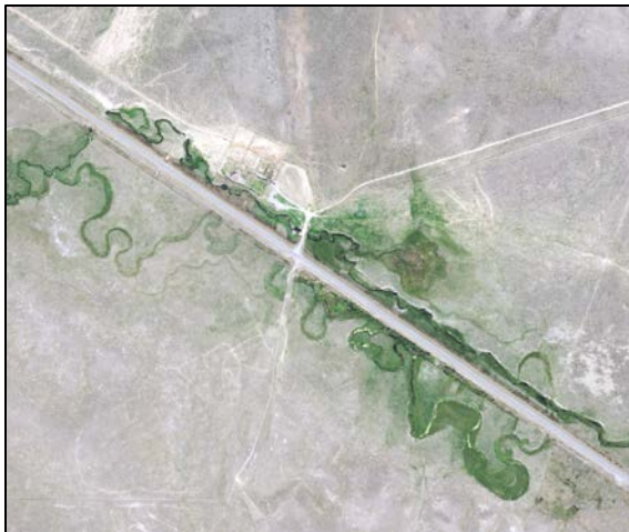
Figure 88. Channelization of the South Fork River due to Highway 89 and railroad grade construction.
