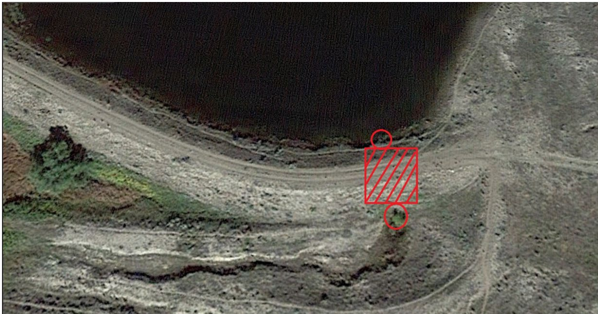
Figure 4. Inlet and outlet locations (red circles) of trickle tube and excavation and pipe replacement area (red square).
