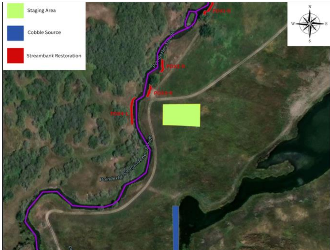
Figure 2. Plan view of the project site including the staging area, cobble source, and four streambank restoration sites. The project will restore ~300' of unstable banks causing excess sediment in the stream.
