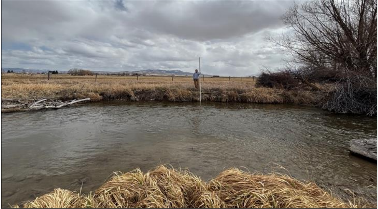
Figure 3. Site PDX1-R (112.68562 °W, 45.17399 °N), a 56.5 ft section of degraded bank with a bank height of 3.1 ft at the midpoint. Site recommendation is to excavate the bank by approximately 9 ft to create a new, sloping floodplain.
