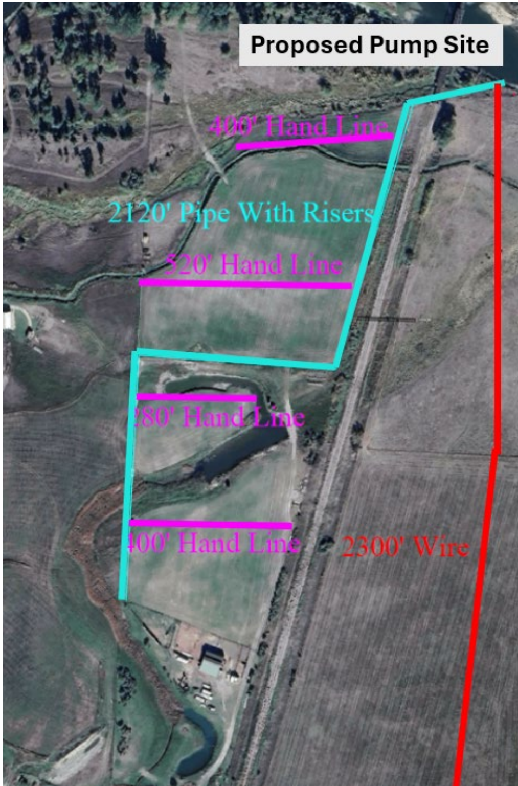
Figure 7. Conceptual design of replacement hand-line irrigation system at Laughery's.
