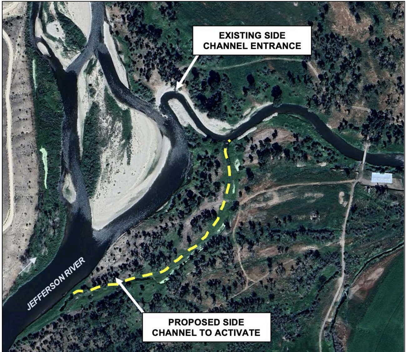
Figure 1: Aerial View of Side Channels
