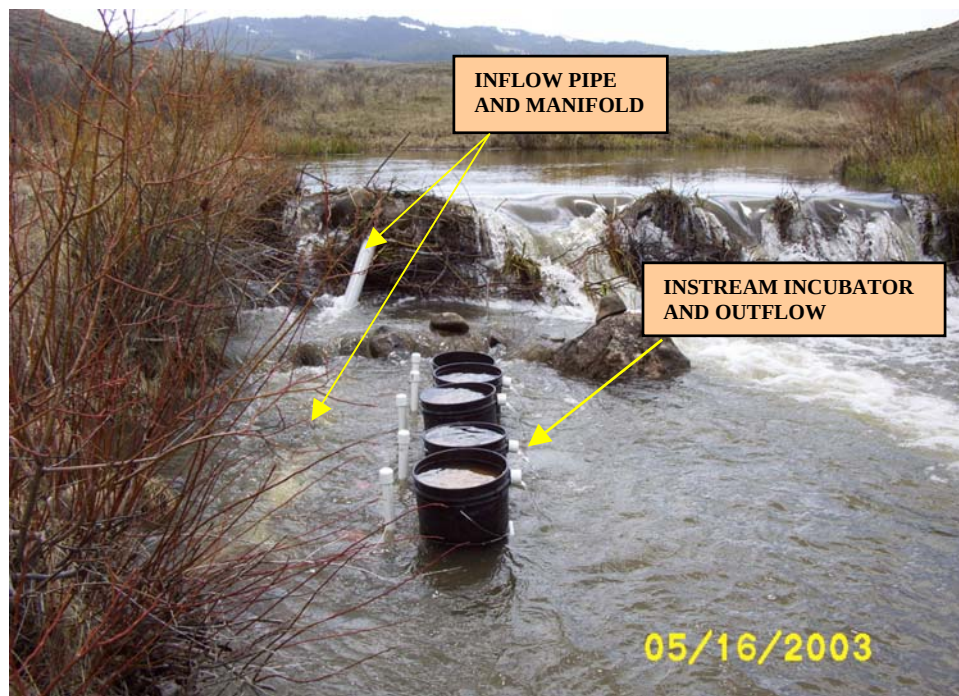
Figure 1. Typical set up for locations with five incubators connected in series.
