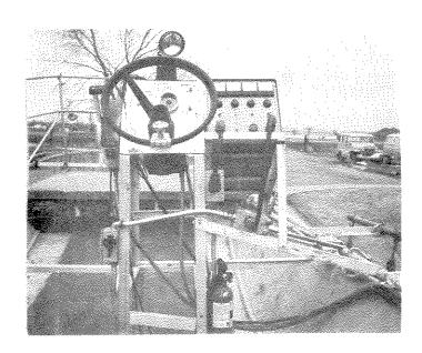
Figure 7. Amphenol screw-lock connectors, waterproof conduit system, and safety switch for boat operator.
