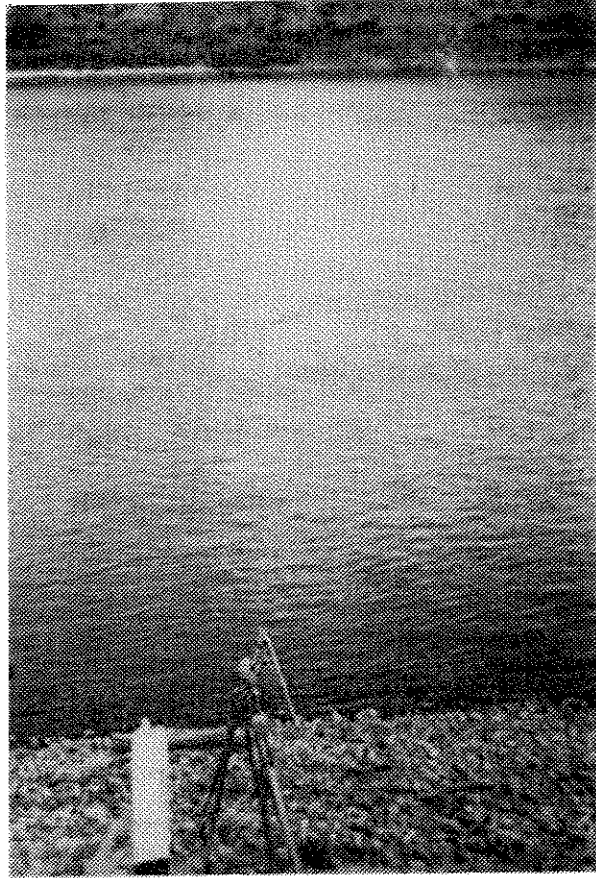
Figure 23. Distances across the channel were measured with a level (foreground) and a stadia rod (far bank). Standard survey techniques were used to obtain elevations between bench marks (steel posts) and a wadable depth (white floats).
