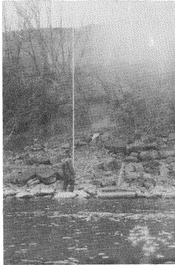
Figure 27. A 7.3 meter collapsible stadia rod was used because of the high banks in many sections of the Yellowstone River.
