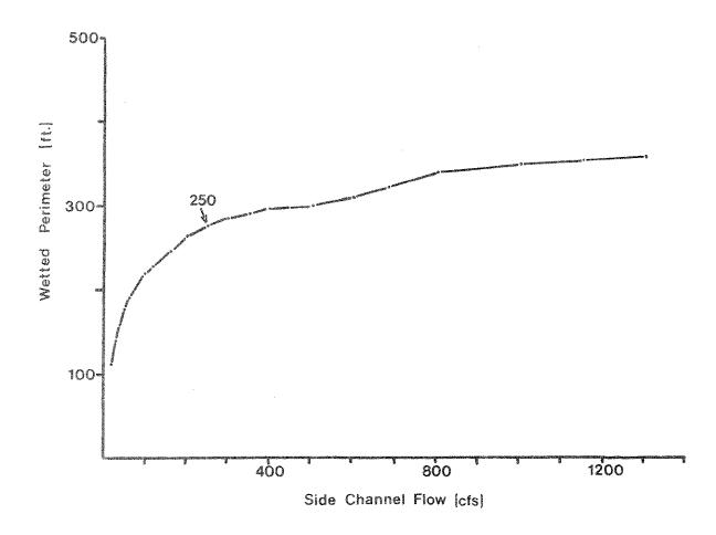
Figure 4. Wetted perimeter-flow relationship for a composite of two riffle cross sections located in the Duck Island side channel of the Missouri River, 1983.
