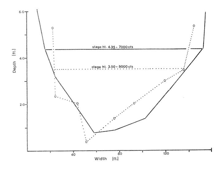
Figure 2. Two cross section profiles of a rearing pool and indicated river stage heights which will maintain the pool at a reasonable condition.
