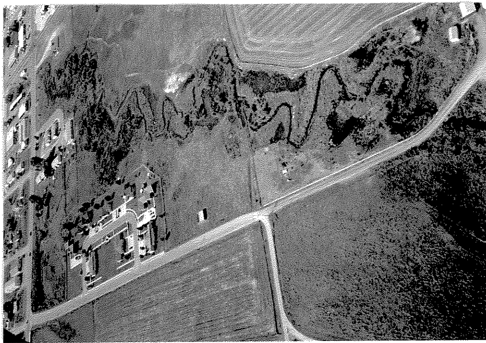
Photo illustration 1. Ronan Spring Creek (located near Ronan) before and after restoration. The channel was narrowed and deepened to restore natural channel geometry, the corridor was fenced and a water gap was constructed to limit cattle access to the stream, and wetlands were constructed adjacent to the stream.
