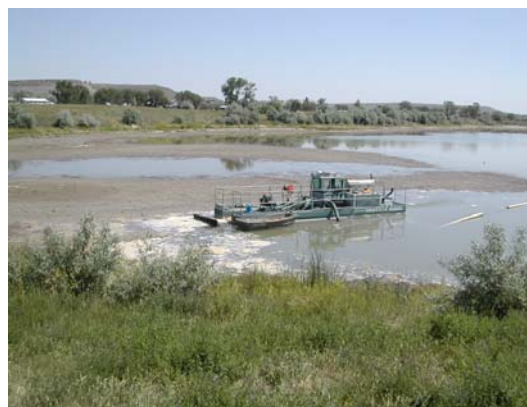
Hydraulic dredge on Wadsworth Pond, near Great Falls.
