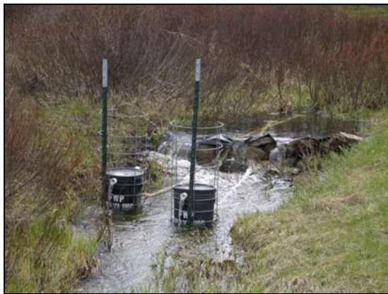
Remote Site Incubators (RSIs) are used in the upper Ruby River to hatch grayling eggs under natural conditions.
