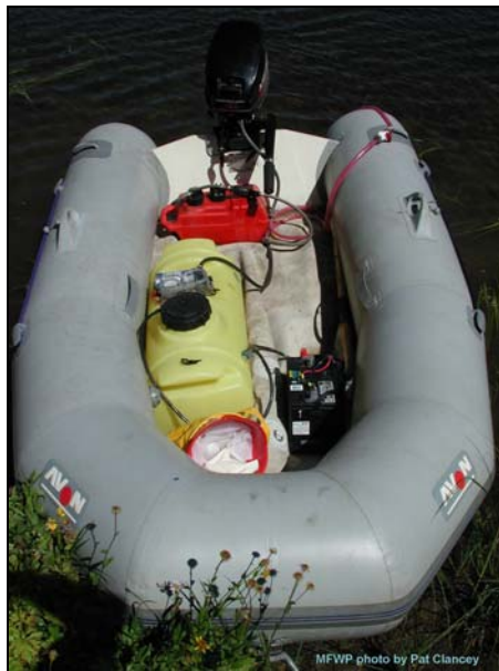
Inflatable raft set-up used to apply Fintrol to Cherry Lake
