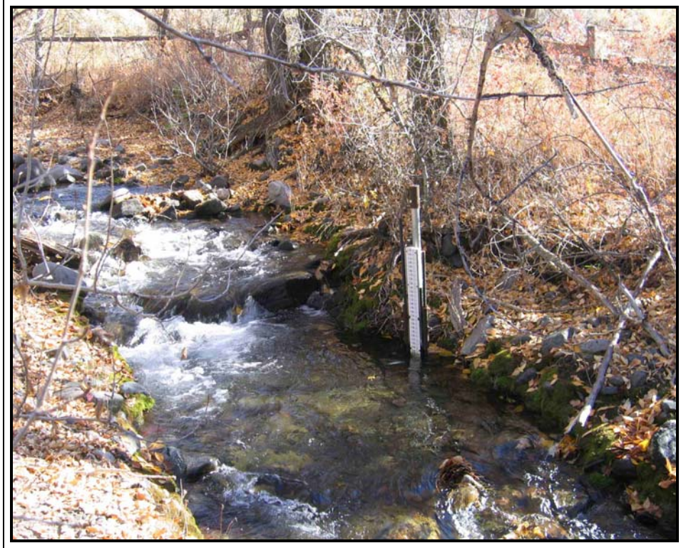
Figure 5. Cedar Creek near mouth. October 26, 2005. The Aquarod® is housed in the metal pipe attached to the staff gauge.
