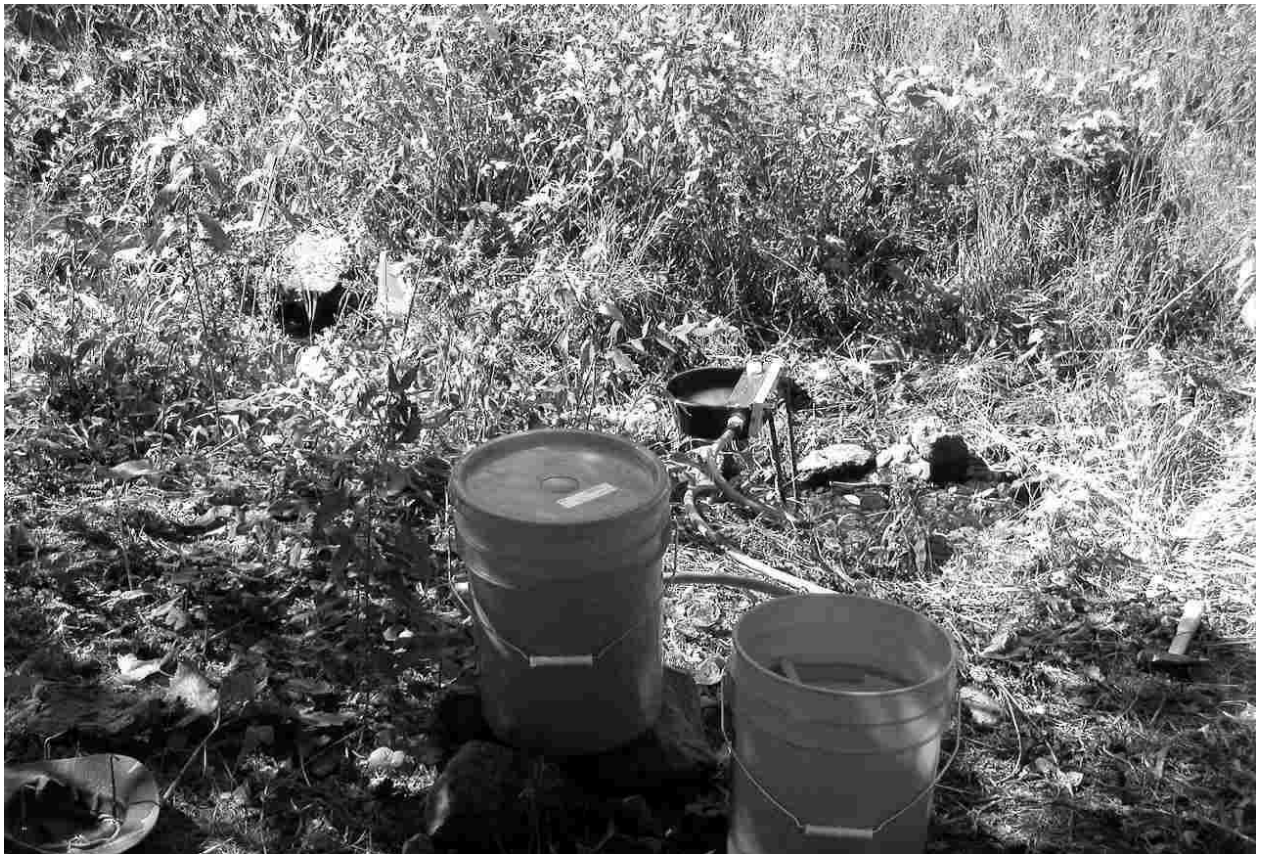
Photo 4. Constant head drip station showing bucket with diluted rotenone and constant head bowl applying rotenone to the stream.
