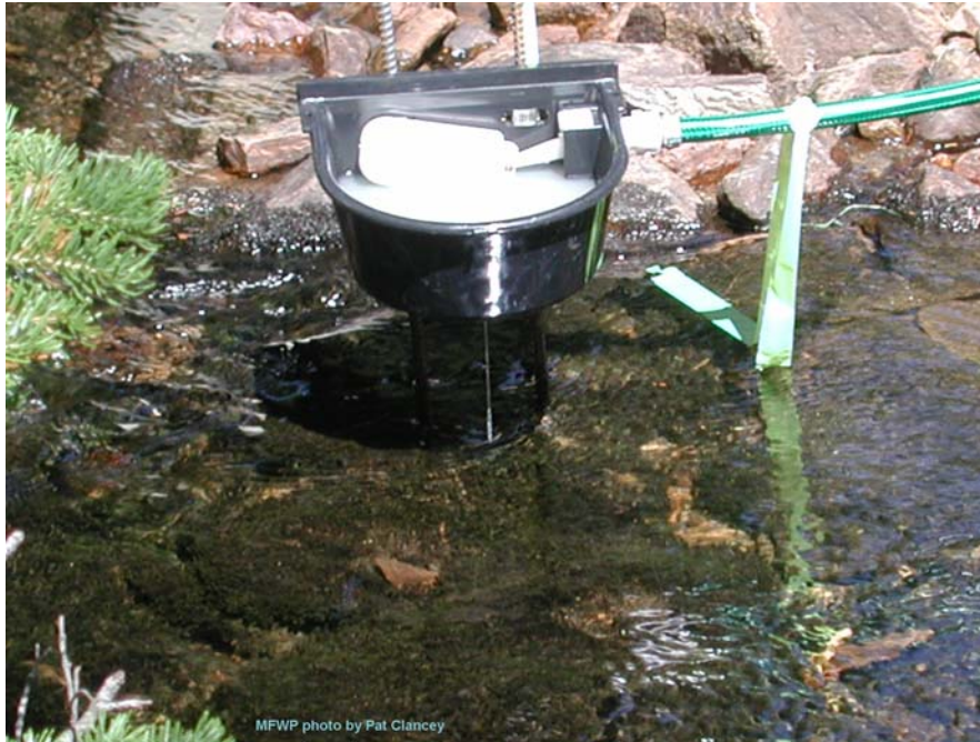
Figure 13. Close-up view of the dog waterer trickling Fintrol mixture into the stream during the Cherry Creek Project.
