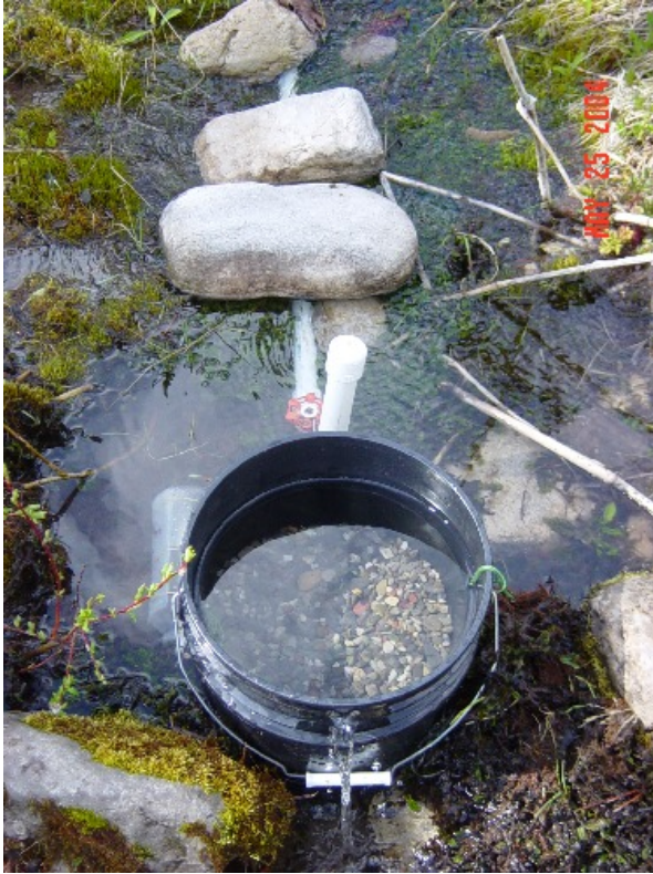
Figure 5-2: Remote site incubator used to imprint fry on a natal stream.
