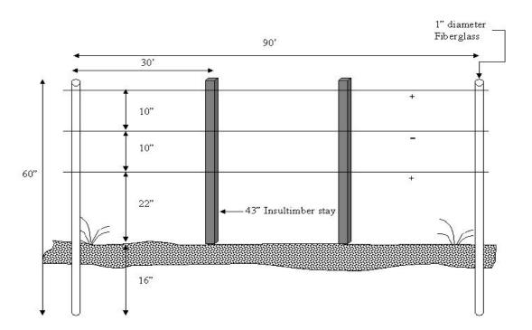
Figure 2. Electric fence design detail cont.
