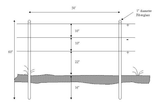
Figure 2. Electric fence design detail cont.
