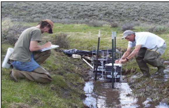
Remote Site Incubators (RSIs) are used in the upper Ruby River to develop grayling eggs to under natural selective mechanisms.
