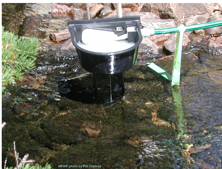
Figure 14. Close-up view of the dog waterer trickling CFT/streamwater mixture into the stream during the Cherry Creek Project.
