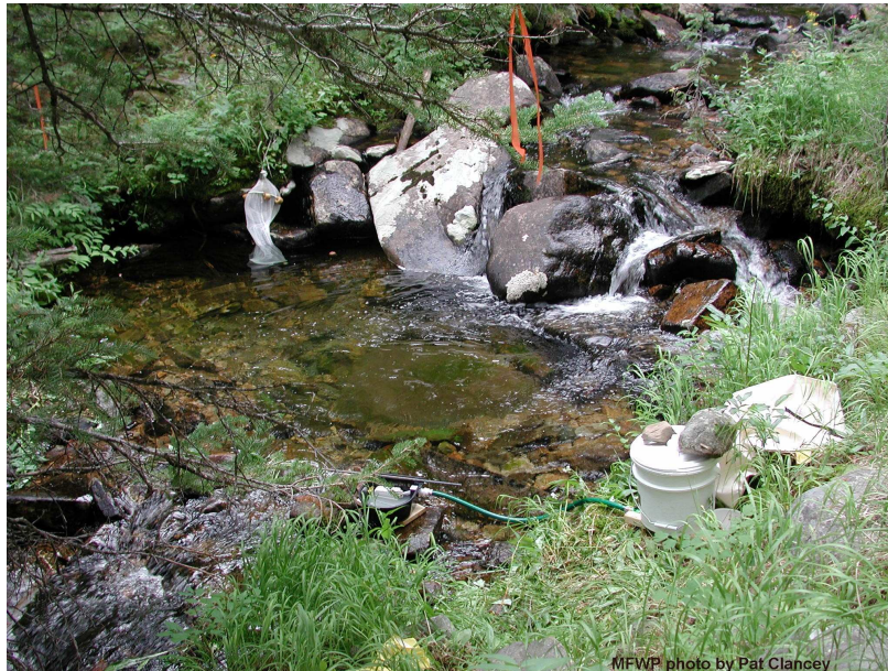
Figure 12. Trickle system and sentinel fish bag on Cherry Lake Creek. The sentinel fish bag is upstream of the CFT application point to monitor the effectiveness of the station above the one shown here.
