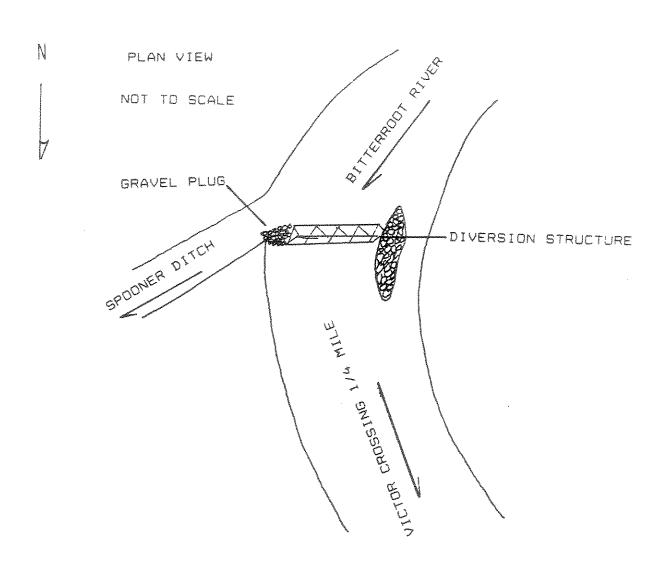
a high point at the junction of the two channels. The diversion structure was placed at the junction, perpendicular to flow in the south channel and parallel to flow in the north channel.
