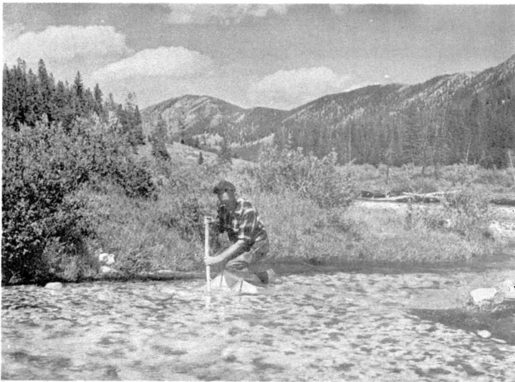
Figure 6. Taking a square-foot stream bottom sample.
