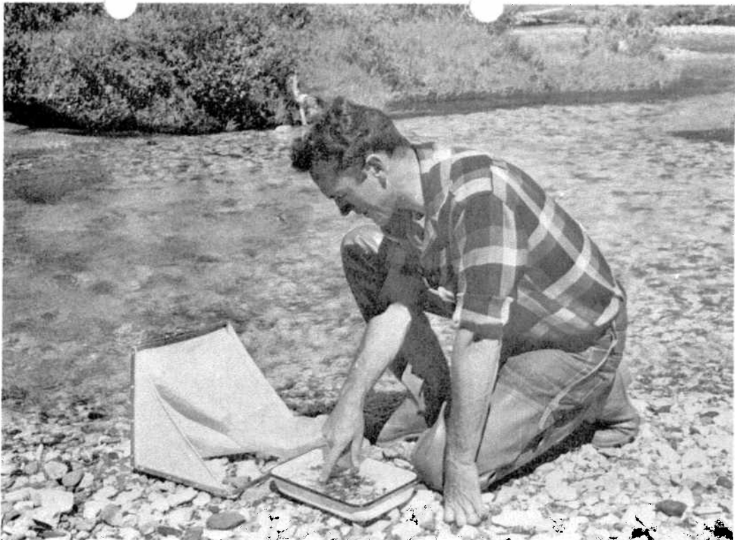
Figure 5. Square-foot bottom sampler with contents in enamel pan for segregation--Canyon Creek.
