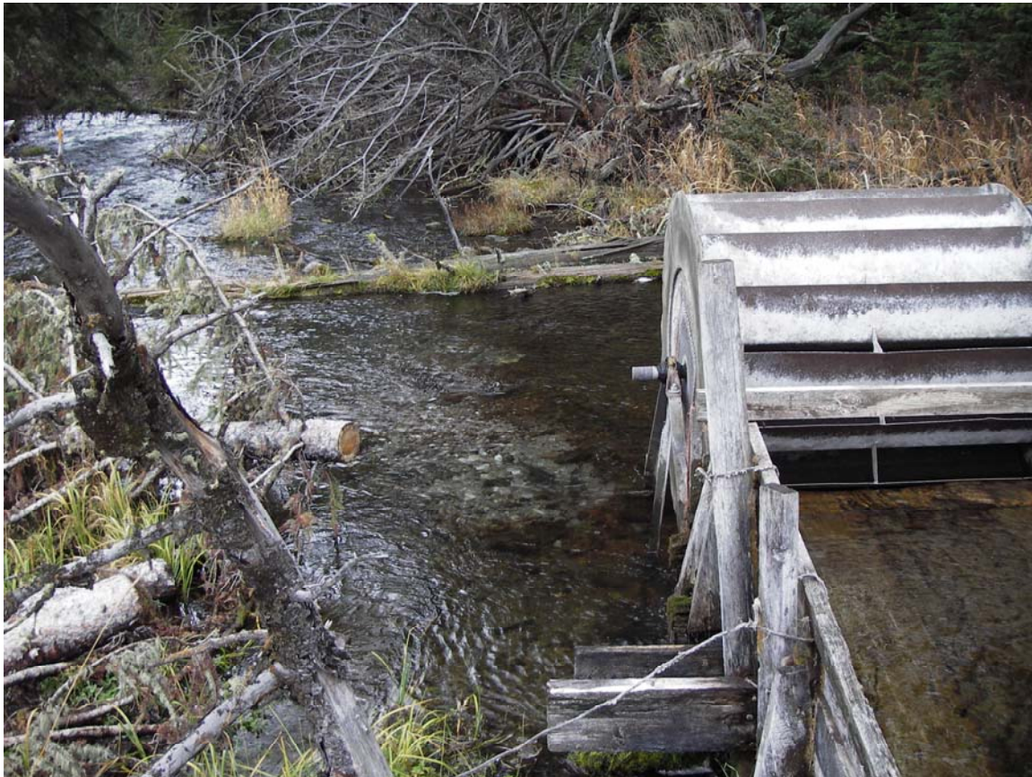
Figure 18. Old water wheel on Lake Creek below Smith Lake compound used to deliver water to cattle during summer months. MFWP photo by Travis Lohrenz.
