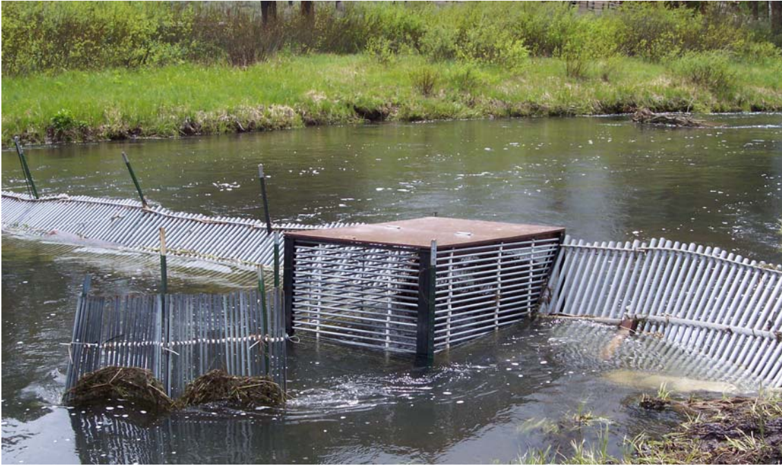
Figure 25. Rigid weir assembly used to trap immigrating rainbow trout on Duck Creek and the South Fork Madison. MFWP photo by Travis Lohrenz.
