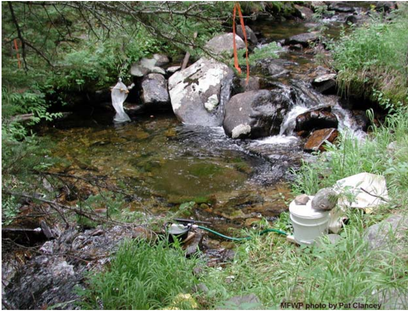
Figure 12. Trickle system and sentinel fish bag on Cherry Lake Creek. The sentinel fish bag is upstream of the CFT application point to monitor the effectiveness of the station above the one shown here.
