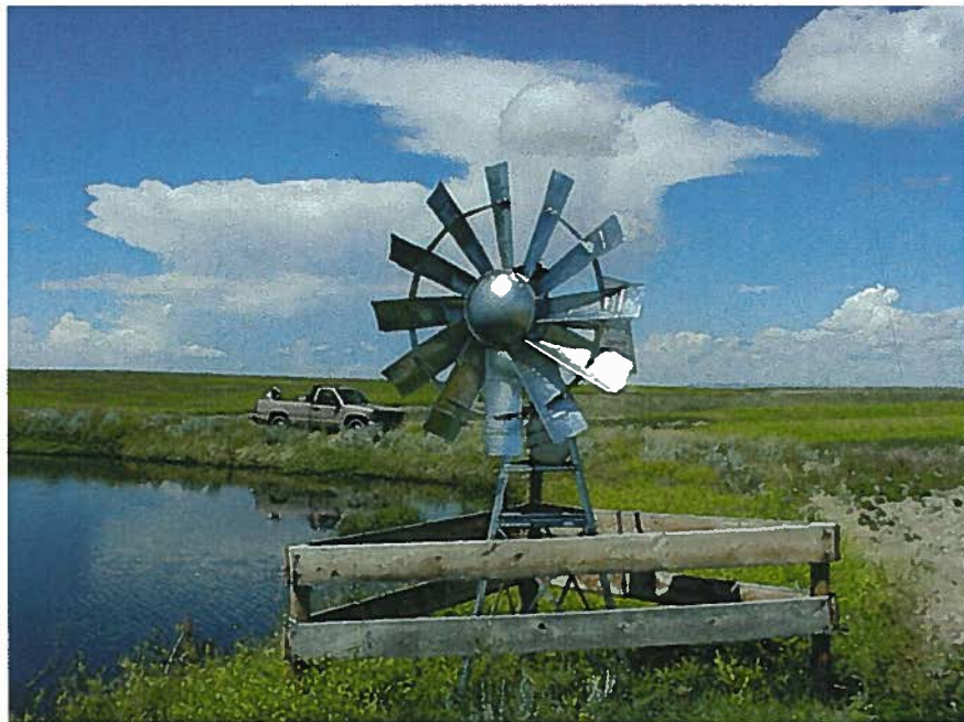
Photo Illustration 5. (Top photo) Installation of a fish screen into a diversion on Little Prickly Pear Creek, a tributary to the Missouri River located north of Helena. Little Prickly Pear Creek is an important spawning tributary for migratory rainbow trout and brown trout from the Missouri River. (Bottom photo) Wind powered aerator installed on Salmo Reservoir located in Blaine County to prevent winter-kill of bass and bluegill.
