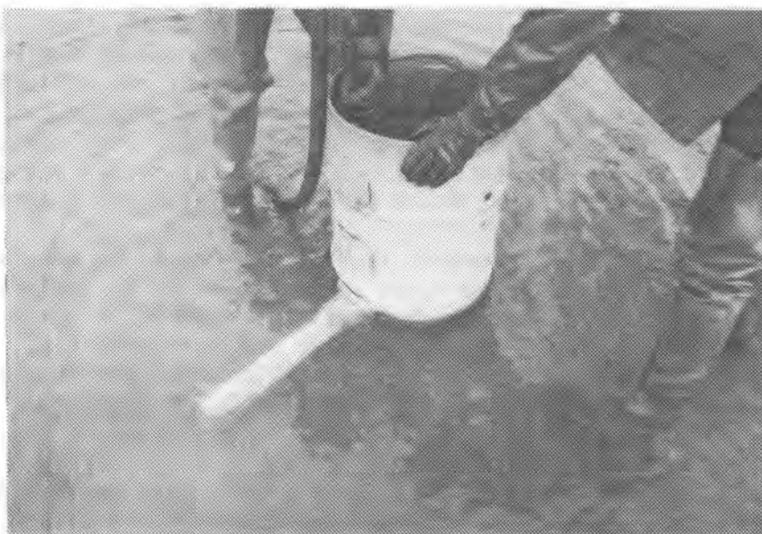
Figure 11. Close-up view of sampler with collecting net attached
