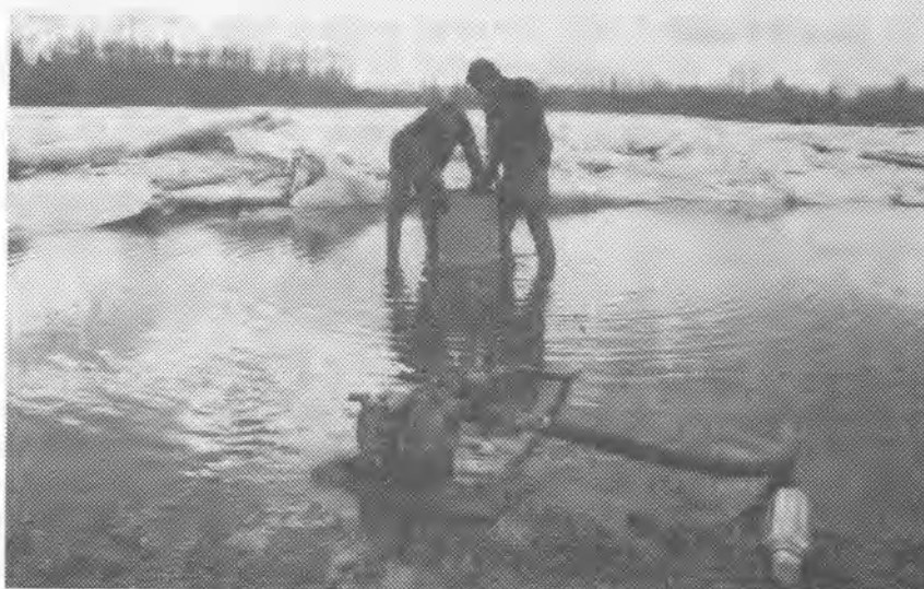
Figure 10. Centrifugal pump and sampler used to collect hydraulic samples of kokanee eggs
