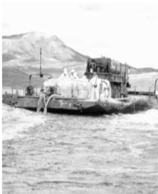
Figure 3.3c Powdered rotenone mixing barges used to treat Strawberry Reservoir, Utah, 1990. Upper figure is a 30-ft barge capable of carrying 4,000 lb of powder. Lower figure is a National Guard ribbon bridge loaded with 24,000 lb of powder.
