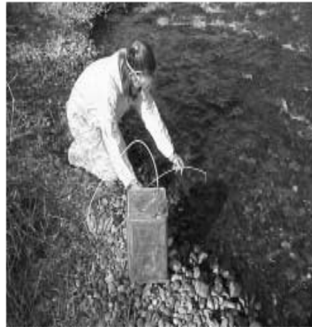
Figure 3.4a Biologist in safety gear calibrating the delivery of rotenone from a continuous drip can into a stream.
