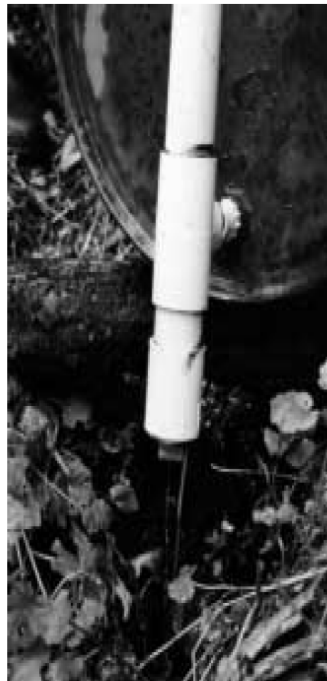
Figure 3.5 Drip barrel system, used by Utah Division of Wildlife Resources, being filled with rotenone and water (top). Drip head dispensing chemical to the stream (bottom).
