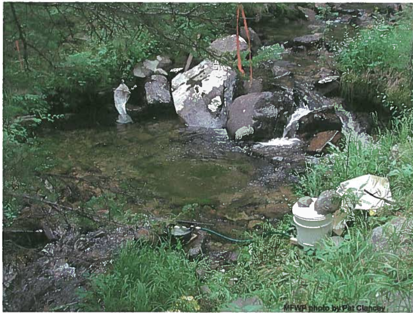
Figure 15. Trickle system and sentinel fish bag on Cherry Lake Creek. The sentinel fish bag is upstream of the CFT application point to monitor the effectiveness of the station upstream of the one shown here.
