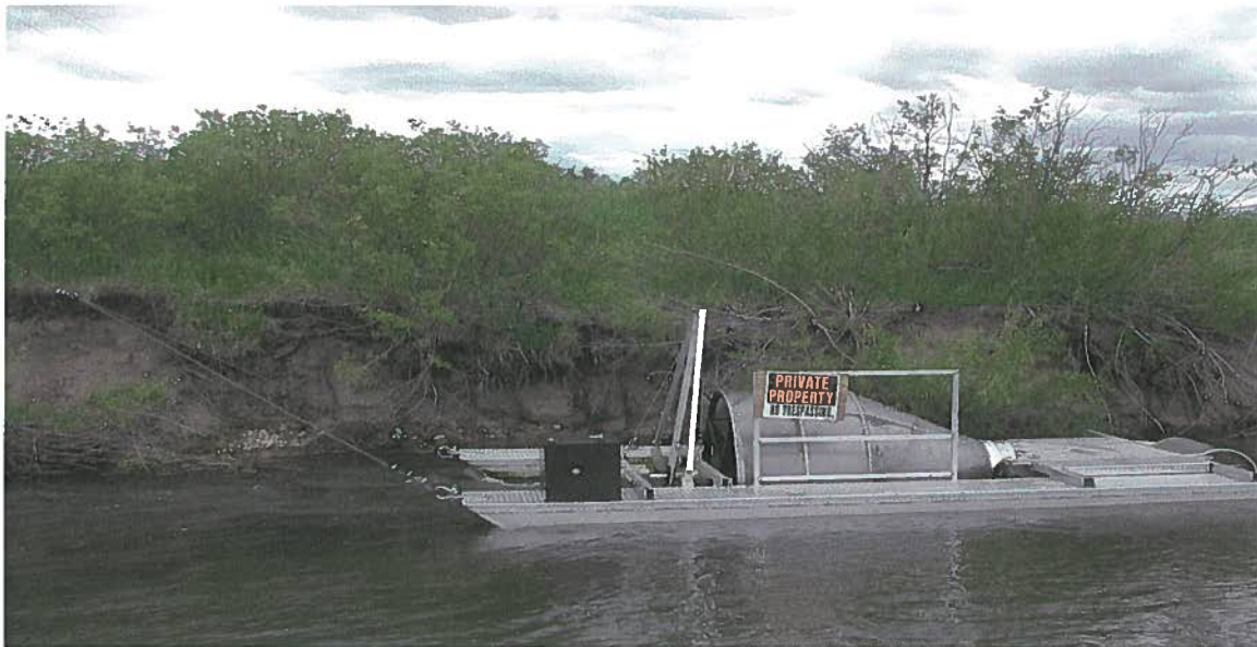
Figure 24. Rotary screw trap used to sample juvenile fish on Duck Creek and the South Fork Madison River.
