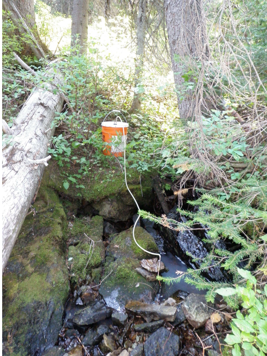
Figure 13. Photograph of a drip station used to deliver the liquid rotenone formulation to the inlet stream to Lower Boulder Lake. Similar apparatus were used on Boulder Creek.
