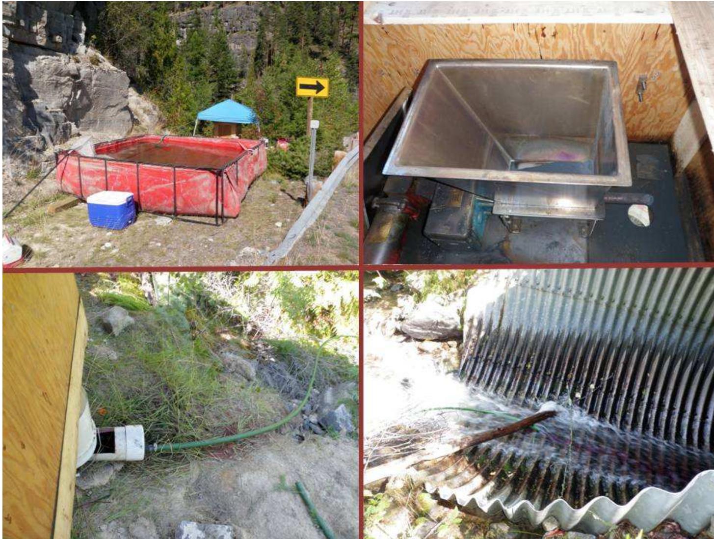
Figure 14. Photographs of the detoxification station used on Boulder Creek located approximately 0.1 miles upstream from Koocanusa Reservoir. The upper left photo shows the water reservoir used to store water used for the water delivery system. The upper right photograph shows the inside of the electric powered auger that metered the potassium permanganate into the water delivery system. The lower two photos show the delivery system used to gravity feed the aqueous solution to the creek.
