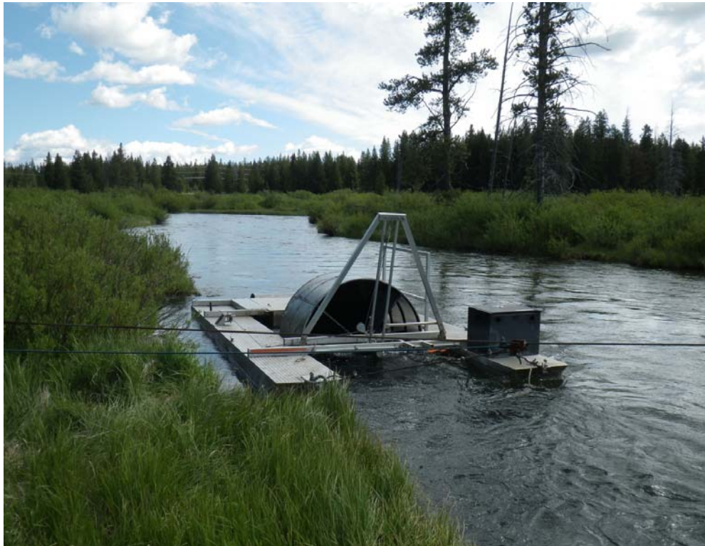
Figure 16. Rotary screw trap used sample juvenile fish on the South Fork Madison River.
