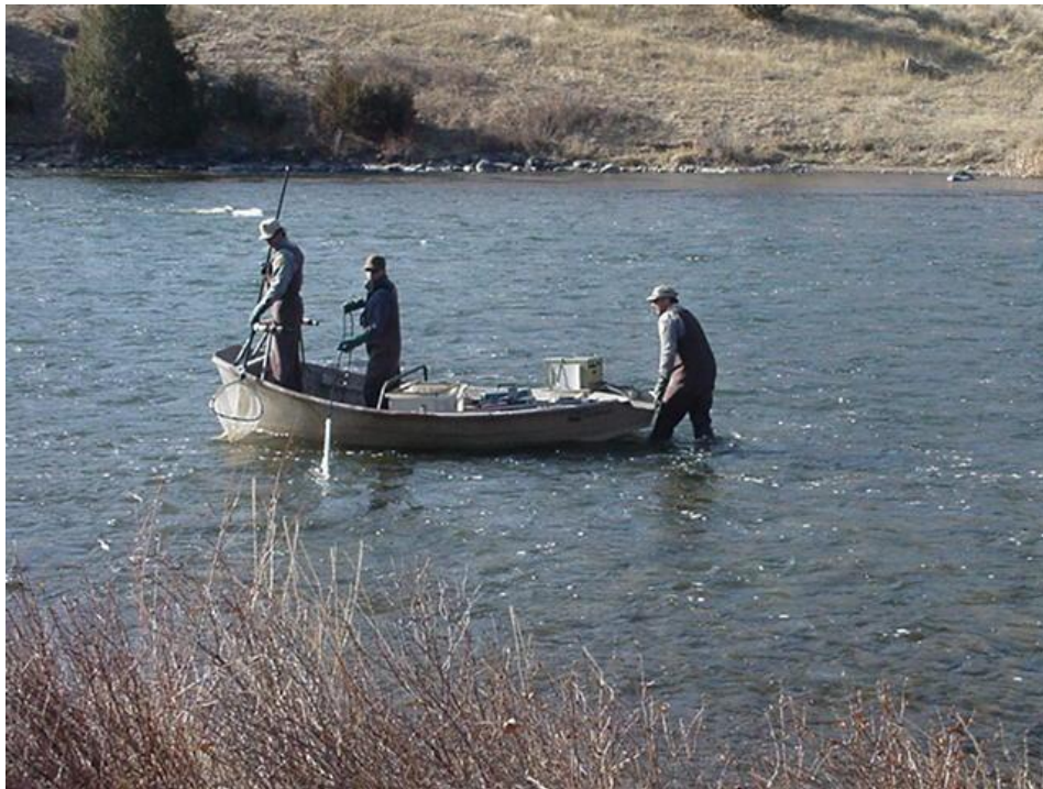
Figure 5. Mobile anode electrofishing (shocking) in the Norris section of the Madison River.
