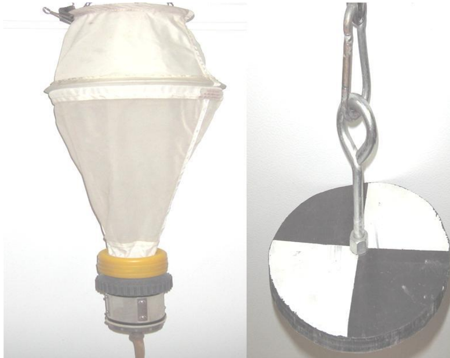
Figure 19. A Wisconsin plankton net (left) and Secchi disk (right) used to collect zooplankton and measure light penetration, respectively, in Hebgen Reservoir.
