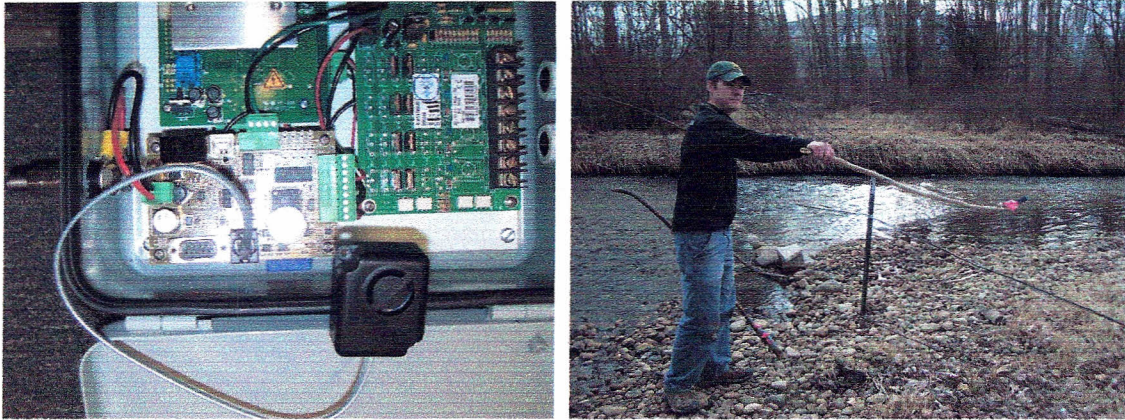
Figure 7a. Pizometer attached to plug-in on Multiplex Reader; and 7b. Testing the detection ability of an antenna. FWP photos.
