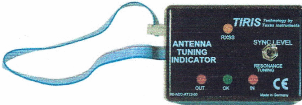
Figure 5. Antenna tuning indicator. Indicator plugs into connector J2 near the corner of the reader board (Figure 4). Photo by Warren Leach, Oregon RFID.
