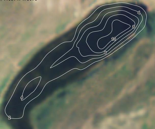
Lake volume and 2 foot contours calculated in ArcMap using 3-D Analyst using GPS survey points from field measurements collected 2015 by Casey Jensen, Region 4, Lewistown. Dawson 1 Reservoir is in Cascade County, Montana.
