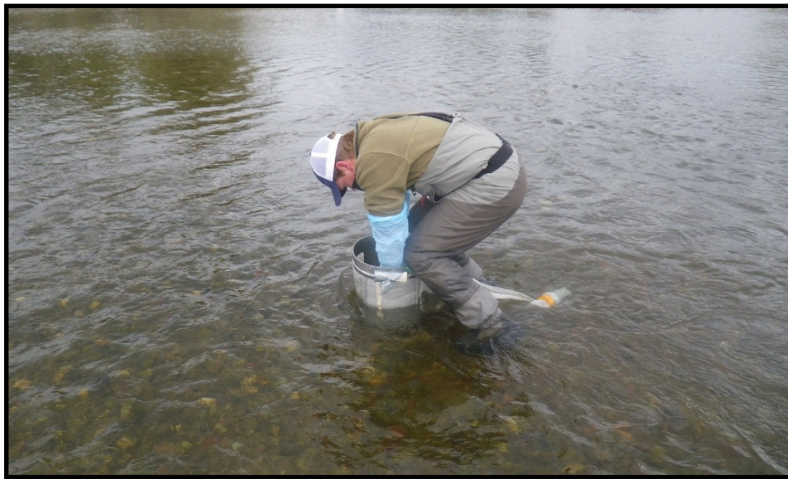
Photo 1. Hess sampling procedure in a riffle of the Missouri River near Little Prickly Pear Creek (MO_LPPC_US).
