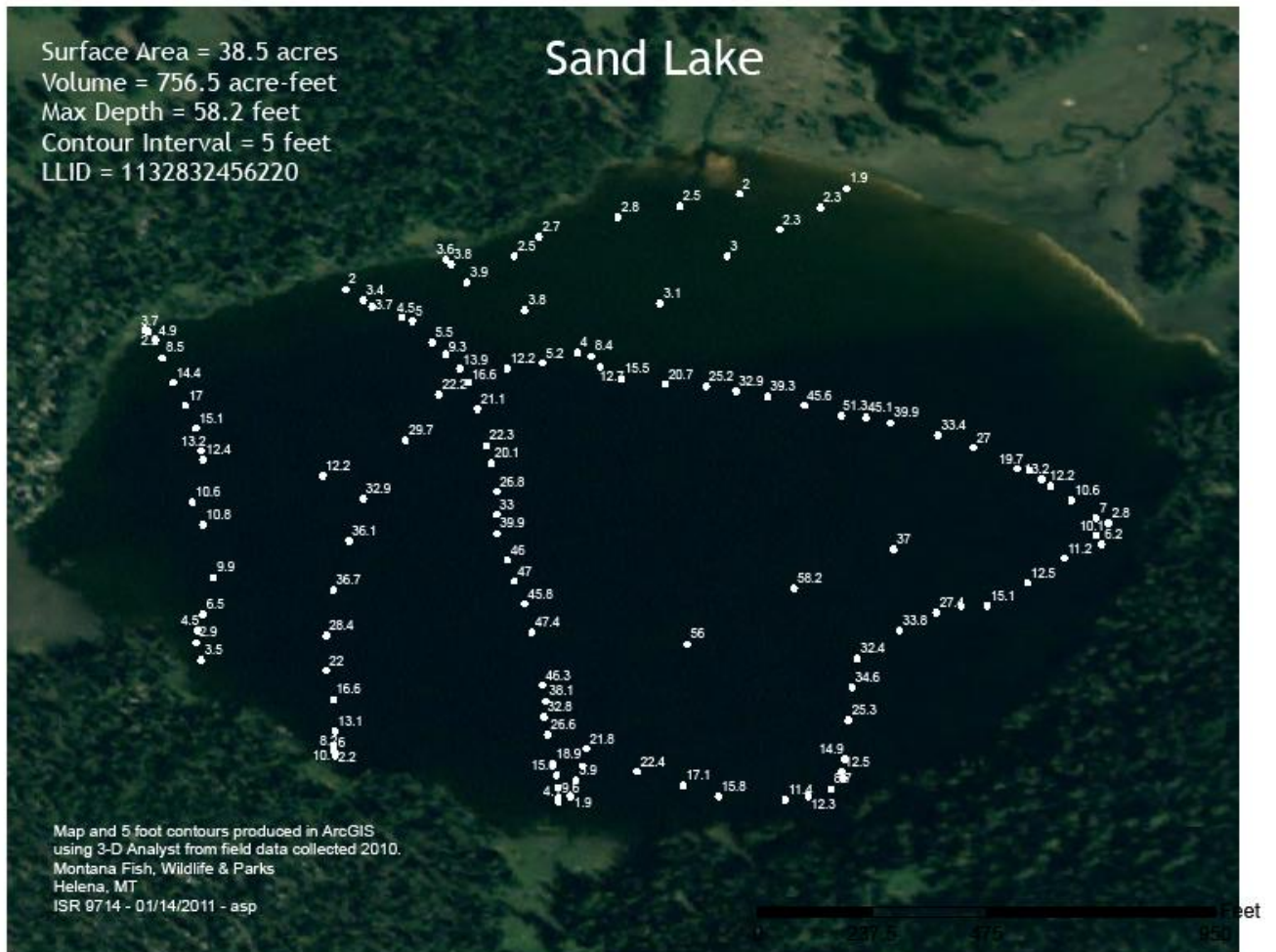
Figure 6. Aerial photo of Sand Lake showing GPS-depth points collected in 2010 and used to generate bathymetric map in Figure 3.
