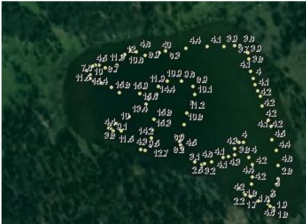
Figure 11. Aerial photo of Granite Lake showing GPS-depth points collected in 2009 used to generate the bathymetric map shown in Figure 10.
