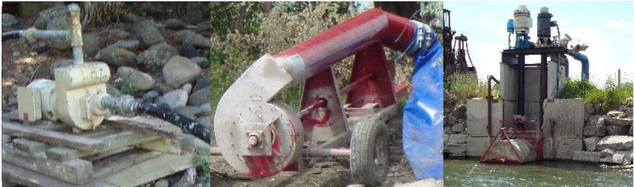
Figure 3.16 Examples of domestic, centrifugal, and turbine pumps.
