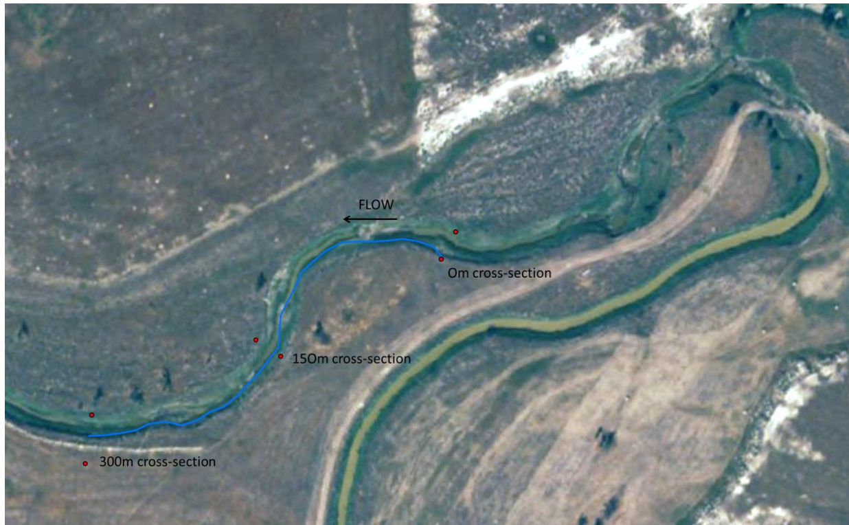
Figure 1. Aerial image of Pumpkin Creek R1. Red dots indicate rebar benchmarks installed on either side of the channel for each of 3 cross-sections. The blue line indicates the 300m sampling reach where fish and habitat surveys were conducted.
