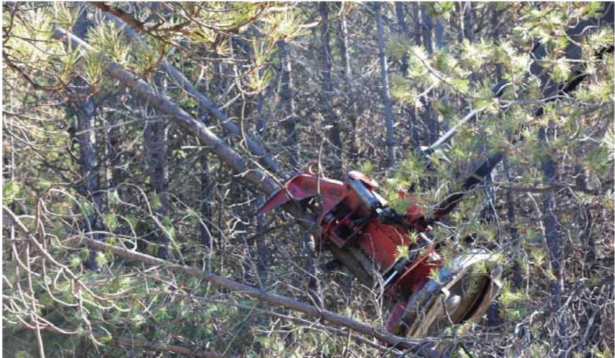
Figure 6. Feller buncher working in a thicket of even-aged ponderosa pine. Almost all of this material was removed to manage the insect and fire risk represented by this anomalous condition that resulted from disruption of the natural fire cycle.
