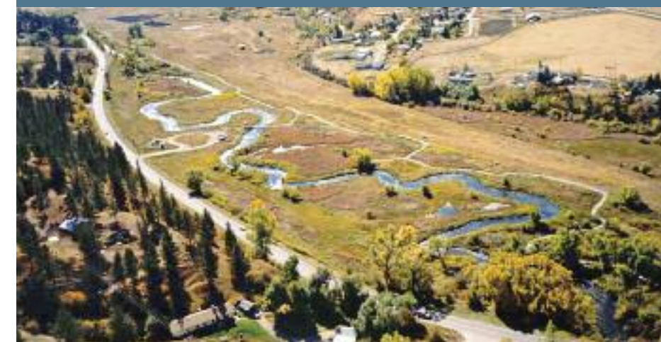
CHANGING CHANNELS Big Spring Creek in Lewistown was channelized in the early 1900s to make room for a railroad line. The above photo shows a later-built road next to the channel, with the original undulating channel still visible. In the early 2000s (below), FWP restored the stream to its historic course, bringing back the curves and bends that produce fish habitat.
