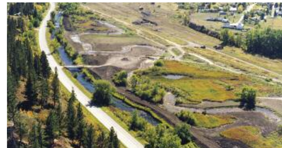
CHANGING CHANNELS Big Spring Creek in Lewistown was channelized in the early 1900s to make room for a railroad line. The above photo shows a later-built road next to the channel, with the original undulating channel still visible. In the early 2000s (below), FWP restored the stream to its historic course, bringing back the curves and bends that produce fish habitat.
