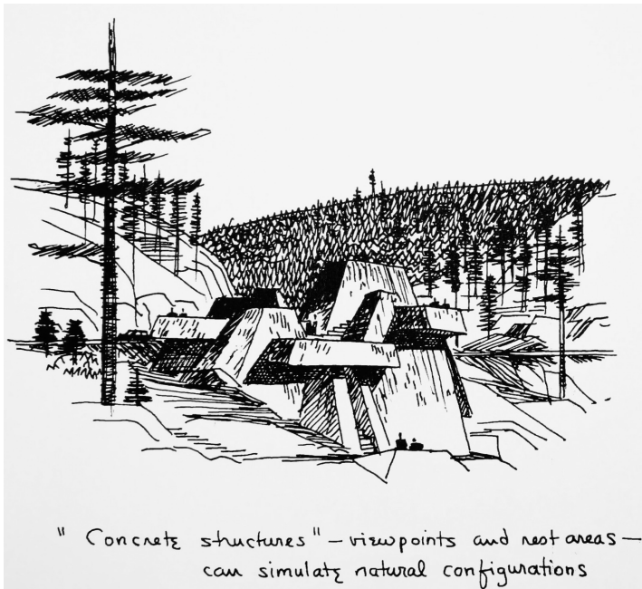
Figure 5. Paul Thiry's "rockscaping" design for the Libby Dam Project's viewpoints and rest areas, using concrete to simulate the mountainous terrain. This type of design was used for other project structures as well, including the dam's powerhouse and visitor center. The original document includes the handwritten annotation. Paul Thiry, Libby Dam Kootenai River, Montana Proposed Architectural Treatment (Seattle, 1965). Used with permission of the U.S. Army Corps of Engineers.
