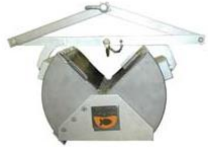
Figure 4: Wildco Ponar Grab Sampler
