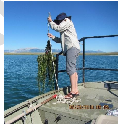
Figure 5 Example of the sampling rake made from a thatch rake with an attached rope.
