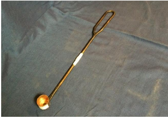
Fig. 9. Bait dispensers are made easily from copper pipe, split rivets, washers, and ¼-inch rod. Match the capacity with a baker's teaspoon. Label the dipper for pesticide use only.
