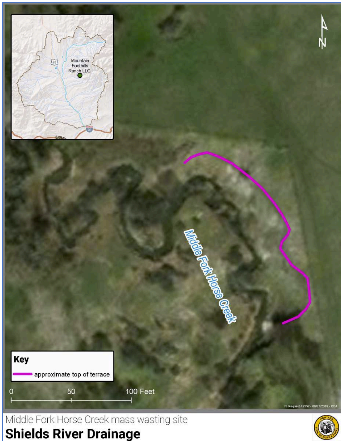
Figure 6. Aerial photo of the area of mass wasting showing the location of the top of the terrace before the event (August 9, 2017).
